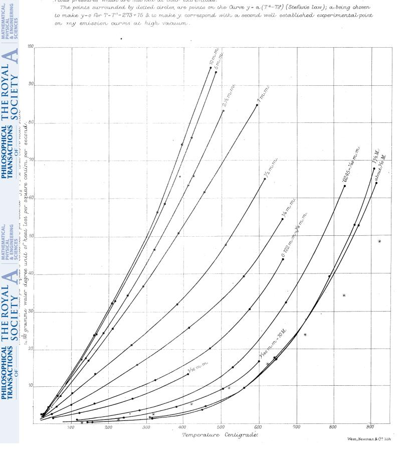
Curve showing for Temperature 408°C. the ratio between the rate of loss of heat with air present at various pressures & the rate of loss at the highest vacuum procurable with the Sprengel Pump the rate of loss at highest vacuum being taken as unity.
